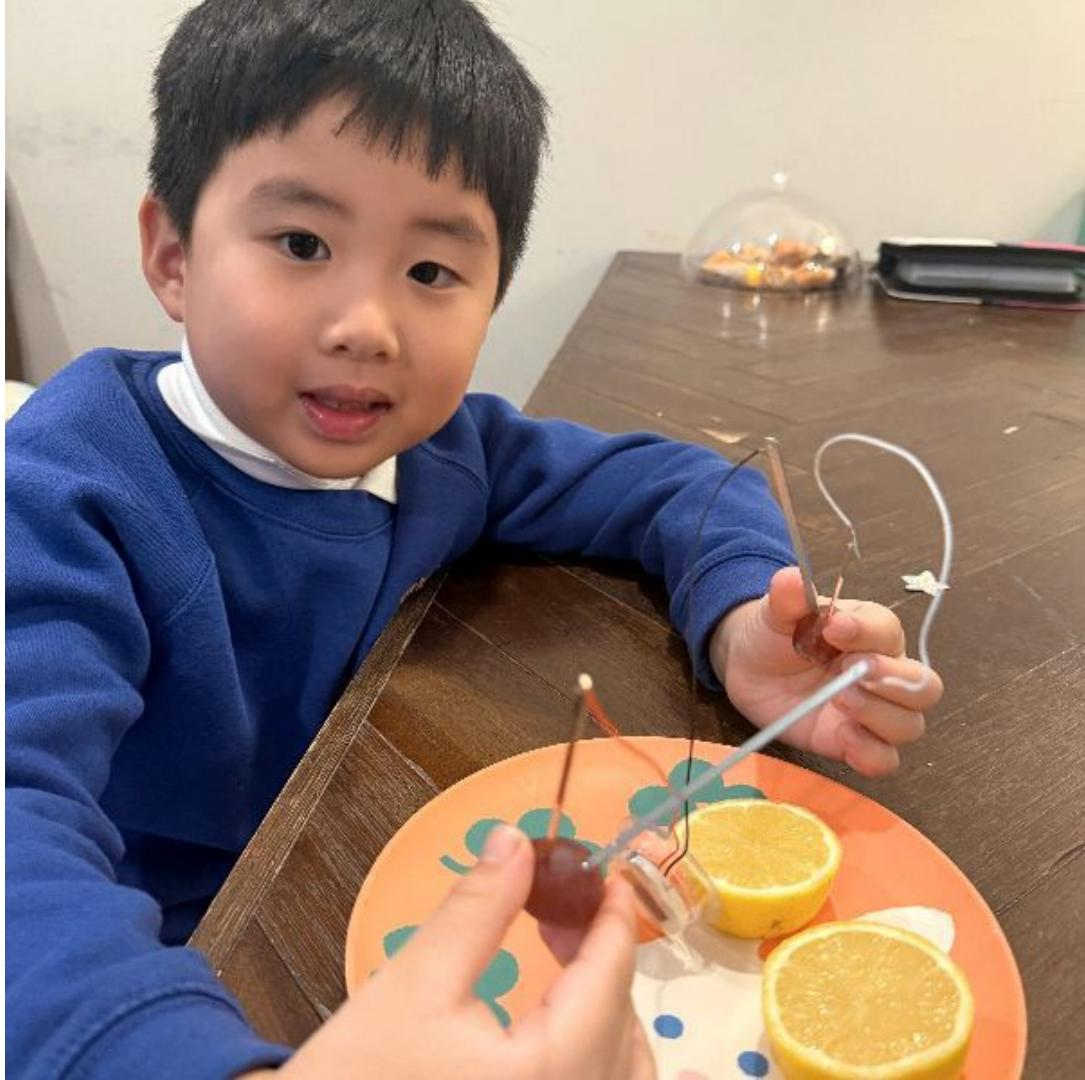
This boy explored how electricity works by making a lemon battery. He inserted copper and zinc electrodes into a lemon and connected them with wires. The chemical reaction inside the lemon created electricity, which was enough to turn a small digital clock on and off. We also learned that grapes can be used instead of lemons to make electricity in a similar way. It was exciting to see electricity made from fruits.
